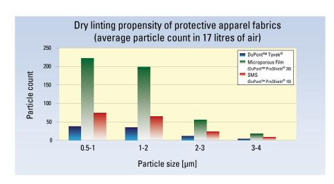
Method for generation and counting of the airborne linting propensity of fabrics in the dry state, BS 6909
